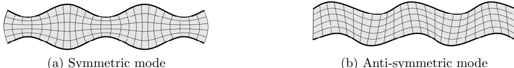
Figure 5: Vibrating modes of an infinitely extent elastic layer. While the symmetric mode corresponds to the thickness stretch motion of the layer where the particle velocity varies through the thickness, the anti-symmetric motion corresponds to the bending and shear motions of the layer where the particle velocity is constant through the thickness.
